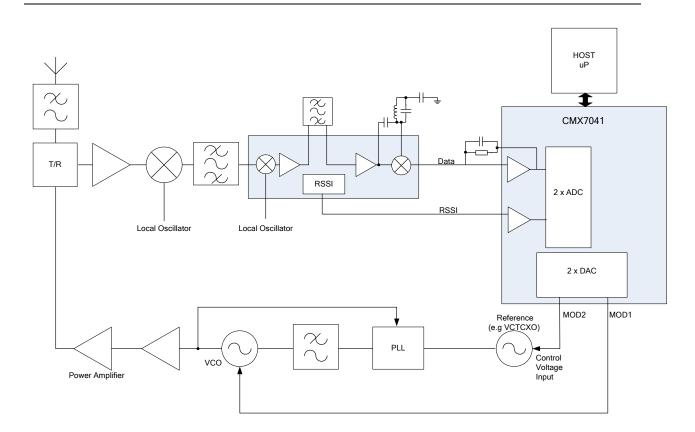
Figure 5 - Radio Transceiver using the CMX7041 implementing two-point modulation
