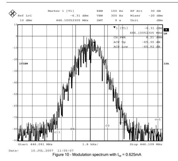
The output is very clean, as would be expected with VCO modulation, the only significant spurii being harmonics. Harmonics will require removal after the power amplifier with a low-pass filter. Results are shown in Figure 11 and Figure 12.
