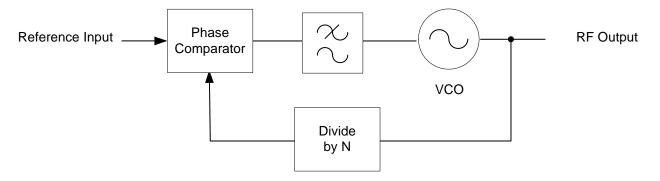
Figure 2 – Phase Locked Loop (PLL)
