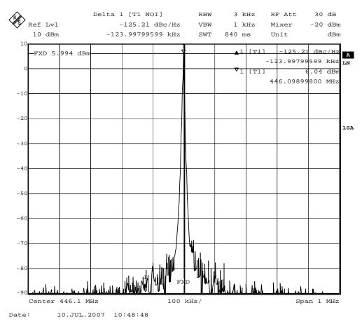
Figure 11 - Modulation spectrum on 1MHz span showing lack of spurious products
