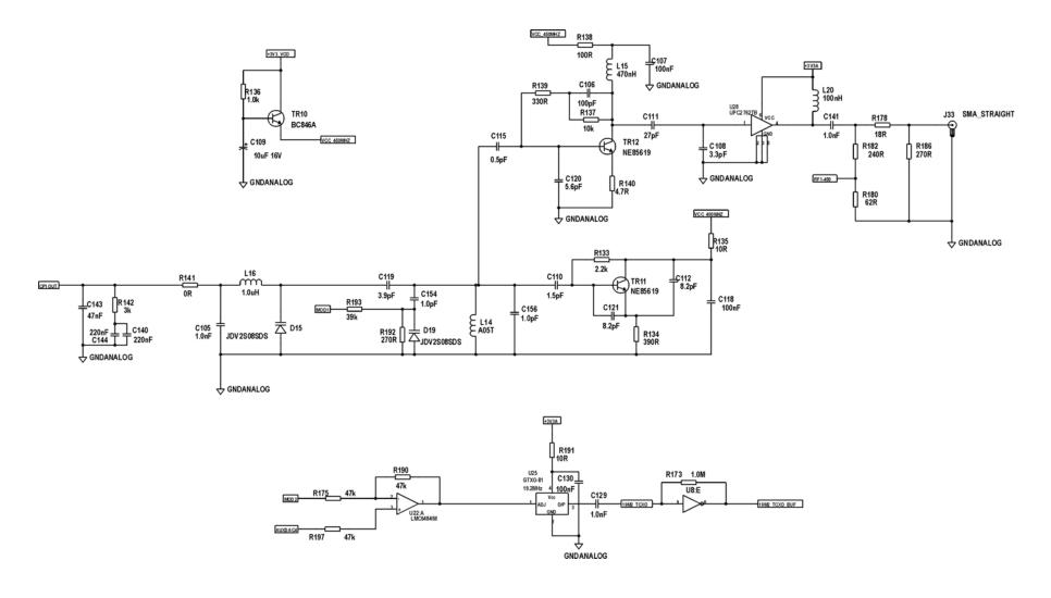
Figure 6 - Schematic of VCO and 2-point modulation circuit
