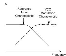
Figure 3 – Modulation characteristics of VCO and Reference modulation in a PLL
