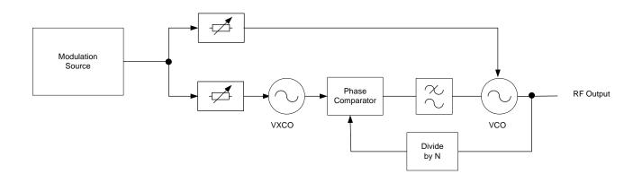
Figure 4 – Two-point Modulation of a PLL
